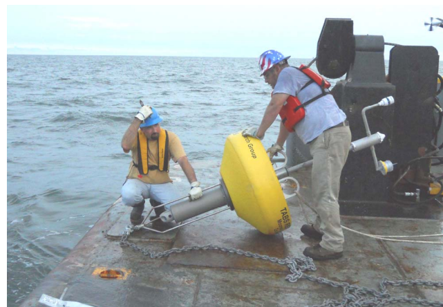
Figure 4: Responder buoy being deployed near Sabine, TX
