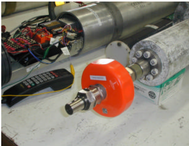
Fig. 5. Acoustic single point Doppler current meter manufactured by Aanderaa. Part of the electronics package from a TABS I buoy is shown in the background. Cellular handset is removed for deployment.
