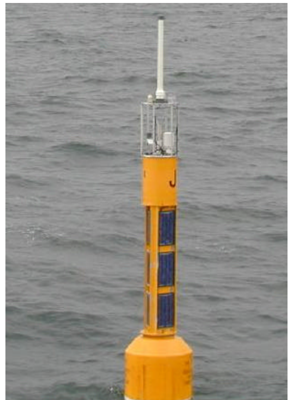
Fig. 3. TABS II Buoy at site J equipped with meteorological instrumentation to measure wind velocity components, barometric pressure and air temperature.
