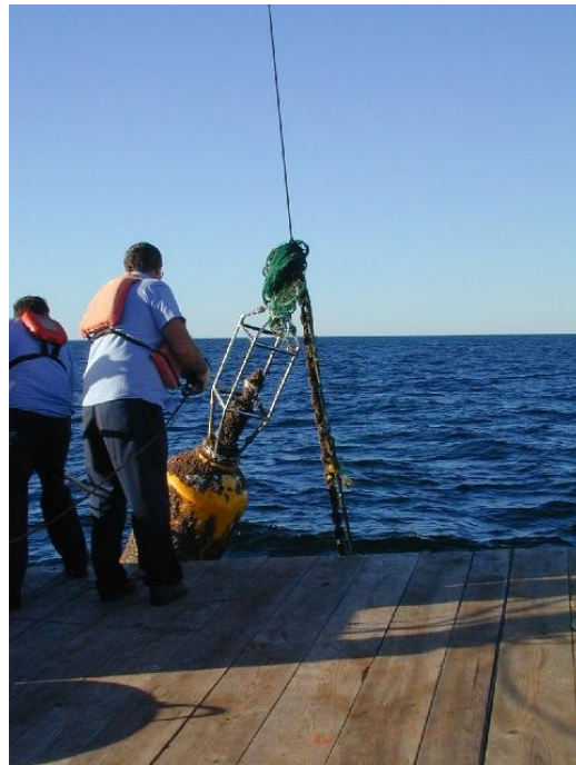
TABS I buoy from site W during recovery with fishing net wrapped around mooring
