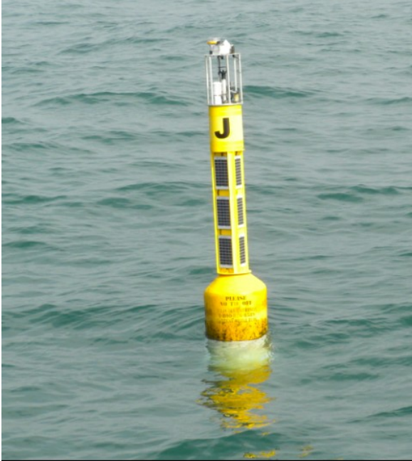
TABS II buoy with meteorological station on top
